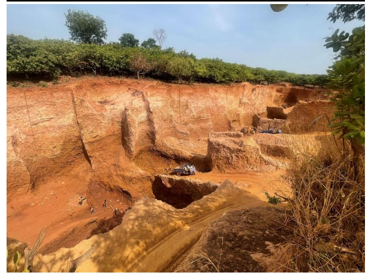
Figure 21: Artisanal mine workings at BMT3
